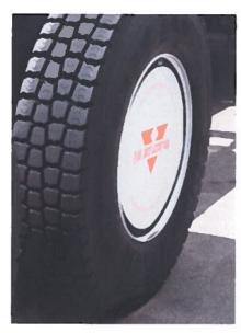
Fitted onto the eight wheels of a truck and its trailer, the Deflecktor cover – made of lightweight fabric – is calculated to cut fuel consumption by two per cent. It works by covering the wheel holes to reduce turbulence as lorries move at speed. Inventor Jon Fleck points out that on industrial-sized wheels, each of the holes is roughly the size of a car window.
